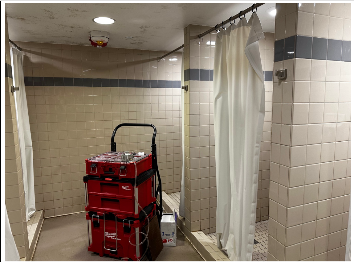
View of testing area – silver unit on top of the hand truck cases is an Anderson Impactor sampler for agar plates.
