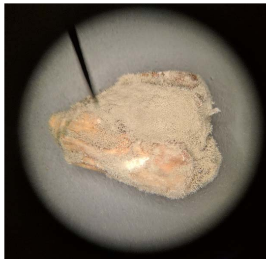
Figure 1. Mold sporulation on sterilized corn kernels. Penicillium brevicompactum is colonizing the kernel in the photograph below. Spores were physically removed from kernels before introduction into the room housing the VentorLux Soulis system.
